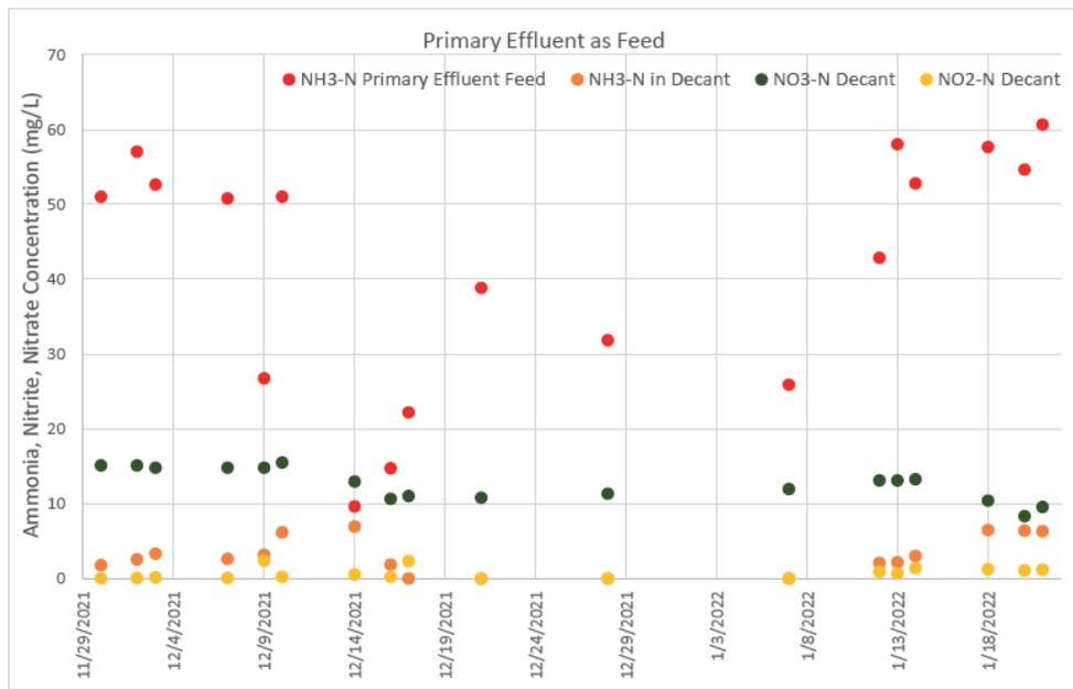
Figure 7: Ammonia, nitrate and nitrite concentrations in MBBR effluent during Experiment 4.
