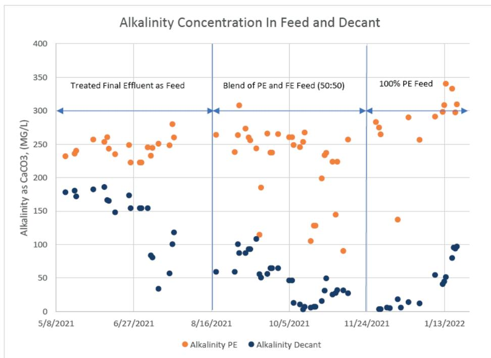
Figure 8: Alkalinity concentrations in MBBR influent and effluent during Experiments 2,3 and 4.
