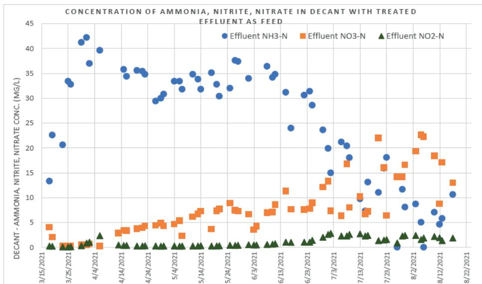
Figure 4: Ammonia, alkalinity, nitrate and nitrite concentrations in MBBR effluent during Experiment 2.
