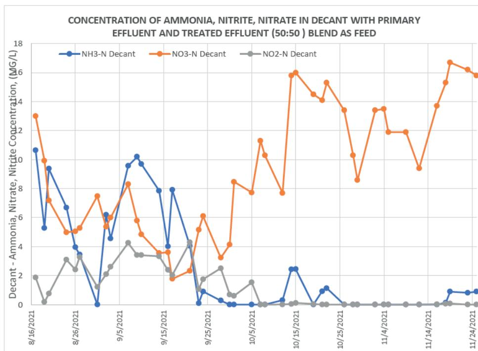
Figure 6: Ammonia, alkalinity, nitrate and nitrite concentrations in MBBR effluent during Experiment 3.
